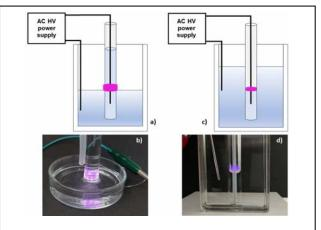
**Fig. 1**. Schematic arrangement and photo of the Open (a, b) and in-tube (c, d) setups of the surface DBD with liquid.#
